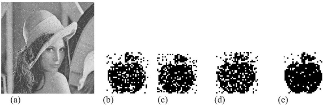
5 'Salt and pepper' noise attack: (a) PSNR=18.2 dB; (b) R channel, NC=0.84; (c) G channel, NC=0.84; (d) B channel, NC=0.82; (e) majority voting, NC=0.93
